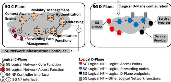
Fig. 4. Examples of 5G core network functions
