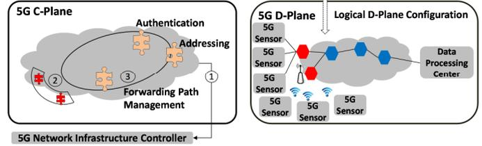
Fig. 5. 5G C/D-Plane for Static/Nomadic Sensors Network Use Case
